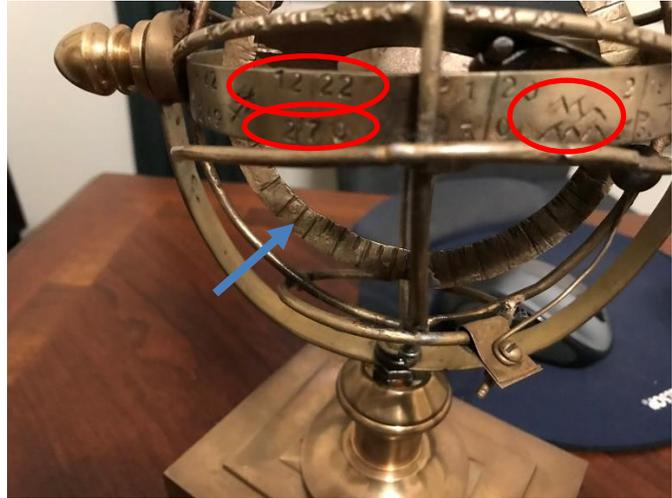
Fig 3 The ecliptic band-date (top red oval), degrees (bottom circle) zodiac (right circle). Also, vertical divisions for each "month". Note the meridian (blue arrow) with its scribed marks.
