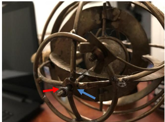
Fig 4 Axis with snap ring (red) and brass square (blue) as guides
