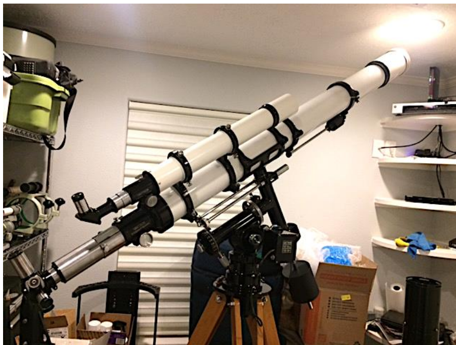
Figure 6. Fully outfitted. This photo shows the scope with guide scope, balance kit, super focuser, and motor drive. The objective almost touches the ceiling, which is 8ft.
