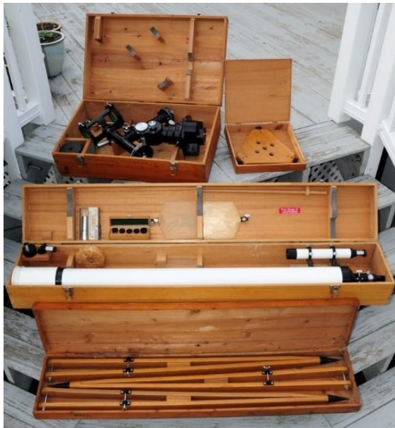
Figure 1. Equatorial mount in case with counterweight storage. Tripod tray in case (Very rare). Optical tube in case with diagonal, porro prism, and eyepiece box. Tripod legs in case.
